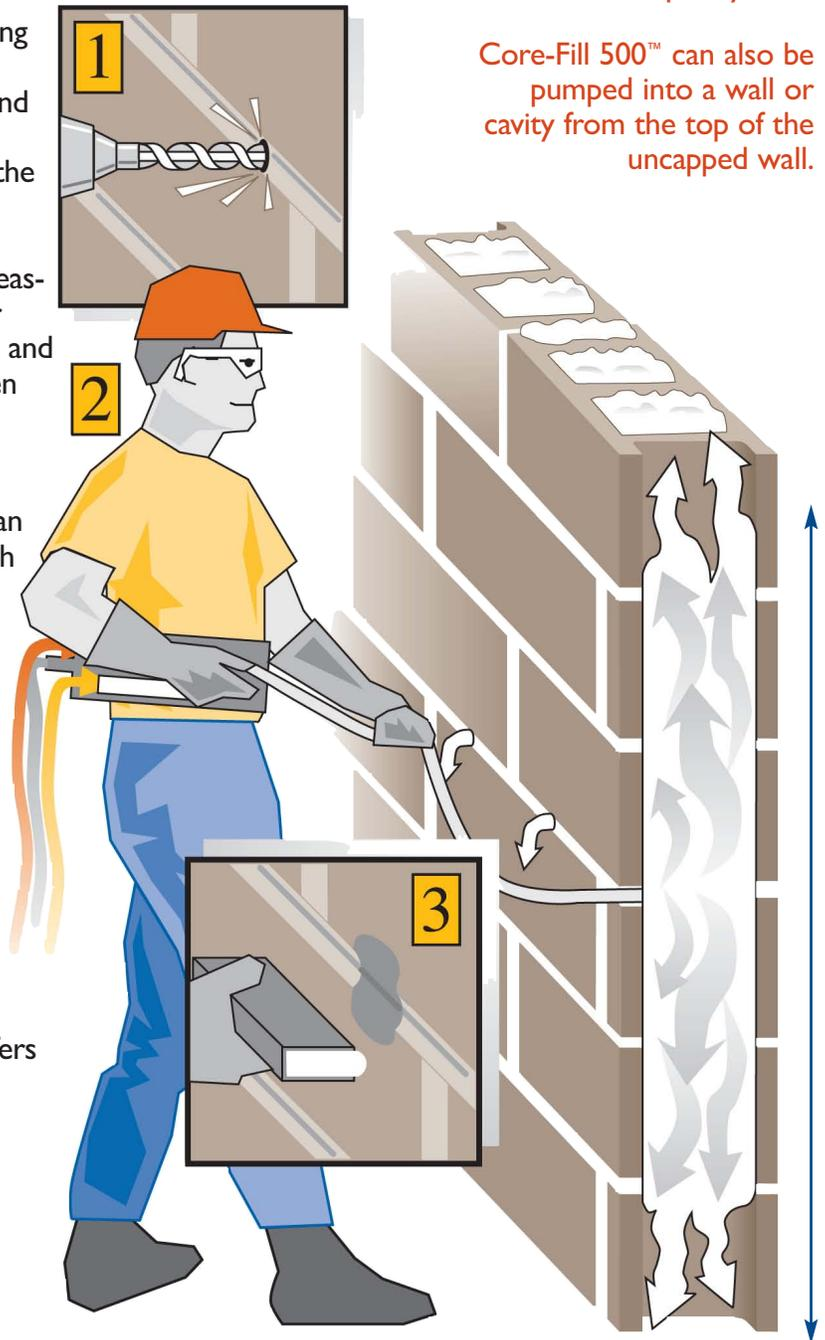
In a typical day, one crew can fill up to 8,000 square feet of wall space with Core-Fill 500™, a speed much higher than alternative methods.
